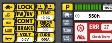
Operation status & fault diagnosis are integrated onto the tiller handle display for easy troubleshooting.
